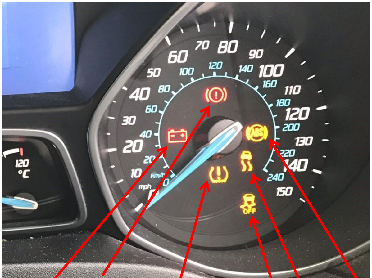
Figure 12. Battery, handbrake on, low tyre pressure,
